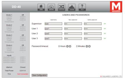
Figure 12 DD-40 web interface – User accounts setup page
