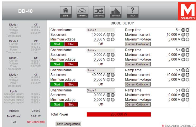
Figure 16 DD-40 web interface – Diode Setup page
