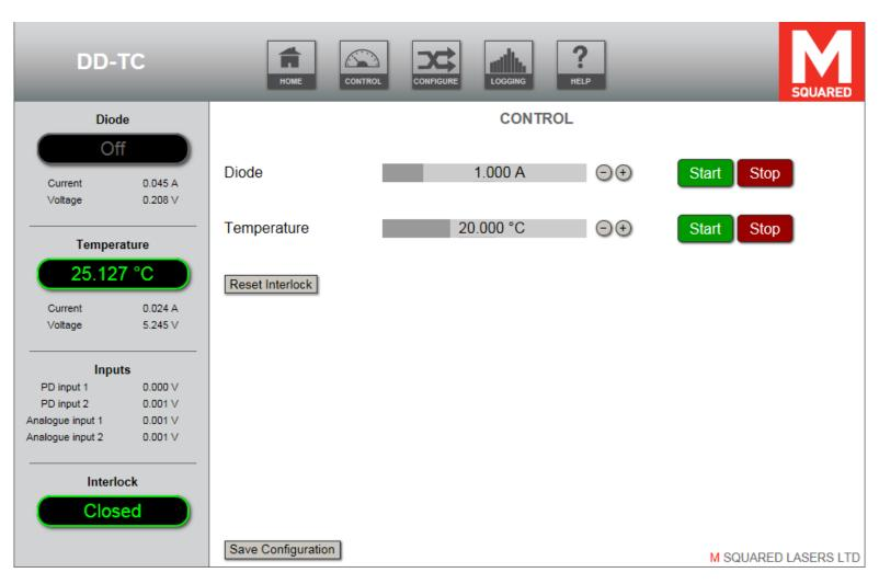
Figure 8 DD-TC web interface – Control screen page
