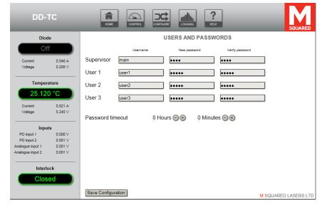
Figure 12 DD-TC web interface – User accounts setup page
