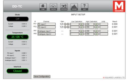
Figure 18 DD-TC web interface – Inputs page
