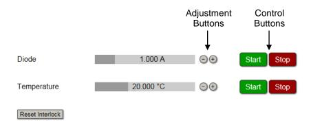
Figure 20 DD-TC web interface – Current and temperature control
