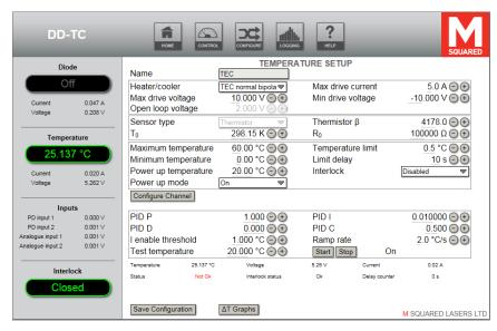
Figure 16 DD-TC web interface – Temperature Channel Setup
